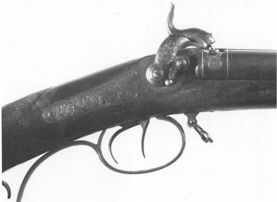
The right hand side of the Stormer shotgun showing the side lock detail. — Los Angeles County Museum of Natural History.
